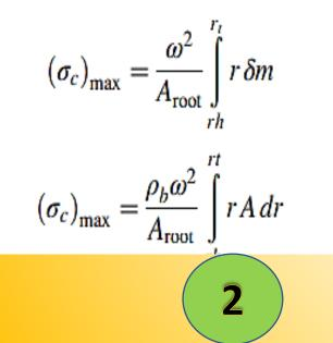
For state of constant area in across of the blade  $\sigma_{max} = 2\pi N^2 \rho_b A$ Where  $A = \pi \left(r_t^2 - r_r^2\right) =$  annulus area  $U_t = \omega r_t = 2\pi N r_t$  $(\sigma_c)_{max} = \frac{\rho_b U_t^2}{2} \left[1 - \left(\frac{r_r}{r_t}\right)^2\right]$
